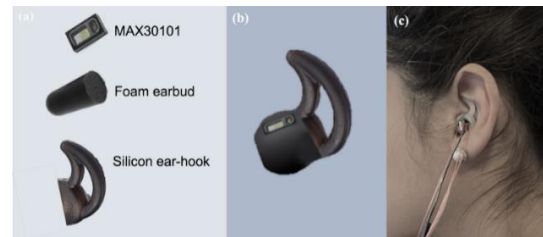
Figure 4. a) Different parts of the in-ear PPG sensor, b) A viscoelastic earbud with a PPG sensor chip inserted in it, attached to an ear hook, c) Placement of the sensor within the ear canal
