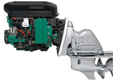
Figure 3. Main engine with a sterndrive (Boatbuy, 2023)
