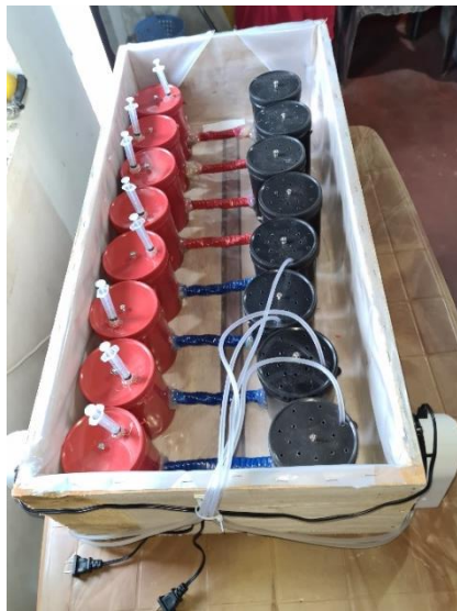
Figure 2 Final MFC 8 Units with all the components attached ready to be tested.
