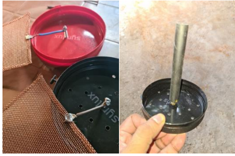
Figure 1 Microbial Fuel Cell Copper & Carbon Electrodes attachment to the Lid
