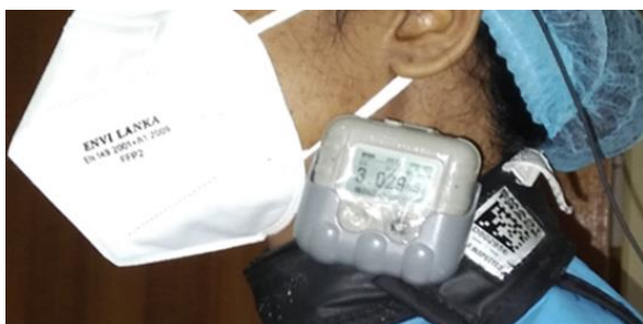
Figure 01: Hp(10) dosimeter positioned above the thyroid collar.
