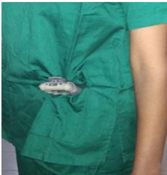
Figure 02: Hp(10) dosimeter positioned under the lead apron
