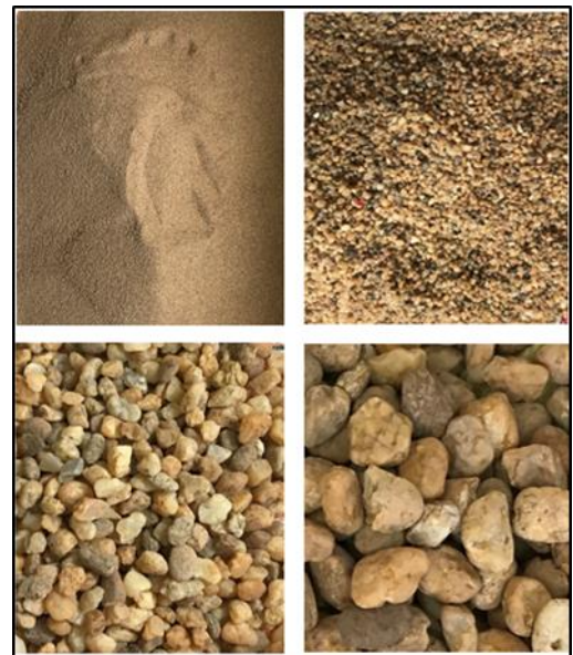
Figure 5: Fine aggregates and gravels as filter media in SSF
