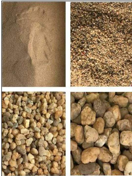
Figure 4: Fine aggregates and gravels as filter media
