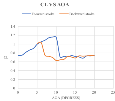
Figure 11. Figure Lift curve for Re = 91412 for forward and backward stroke
