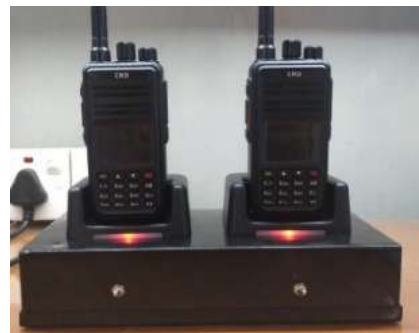
Figure 8. Two-way battery charger for Creeper DMR
