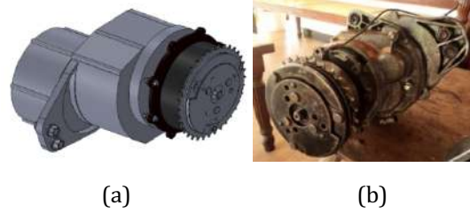
Figure 9. (a) 3D model & (b) motor coupled with EM clutch.
