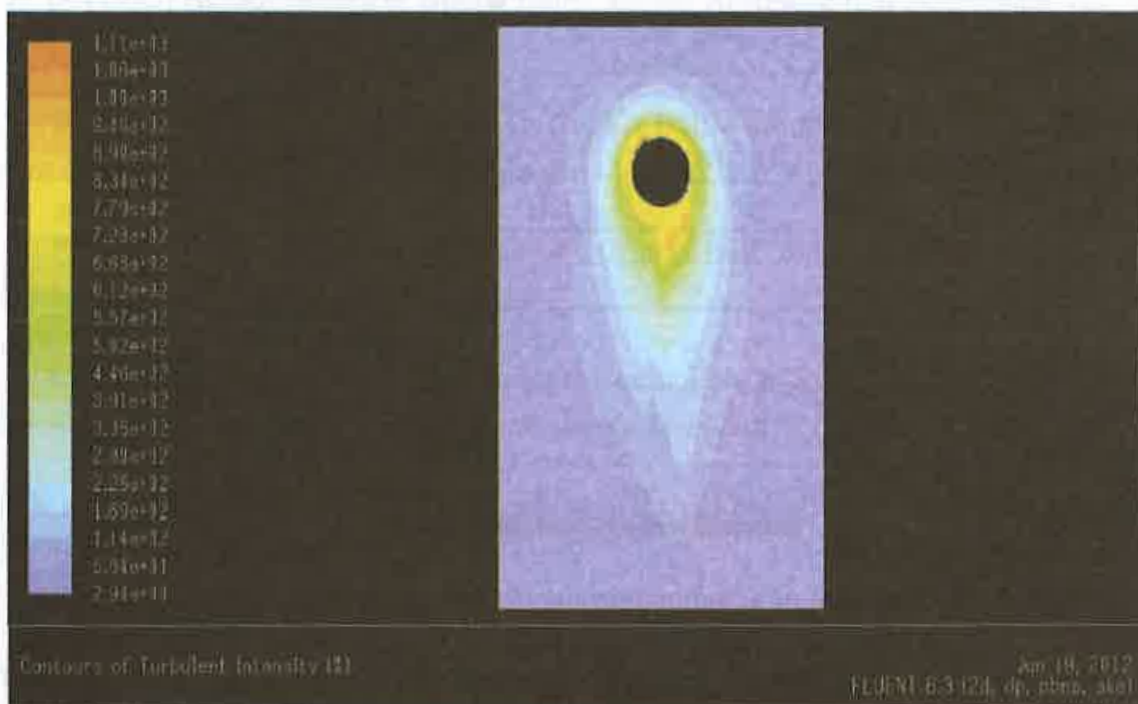
Figure 10: Predicted Turbulent Intensity at seam angle 45^\circ for optimum conventional swing
