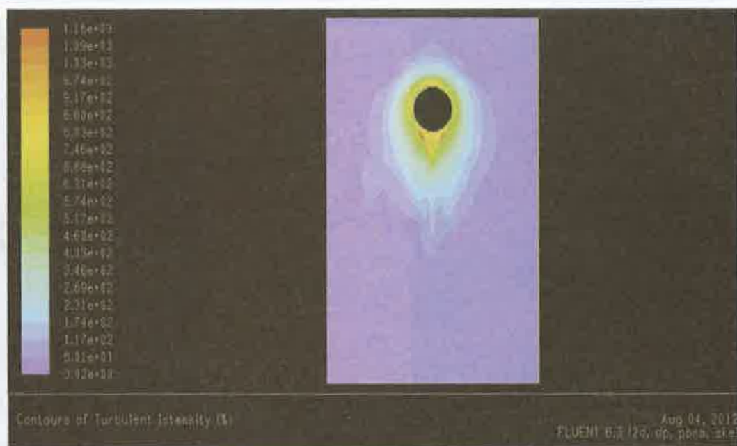
Figure 8: Predicted Turbulent Intensity for seam angle 0^\circ
