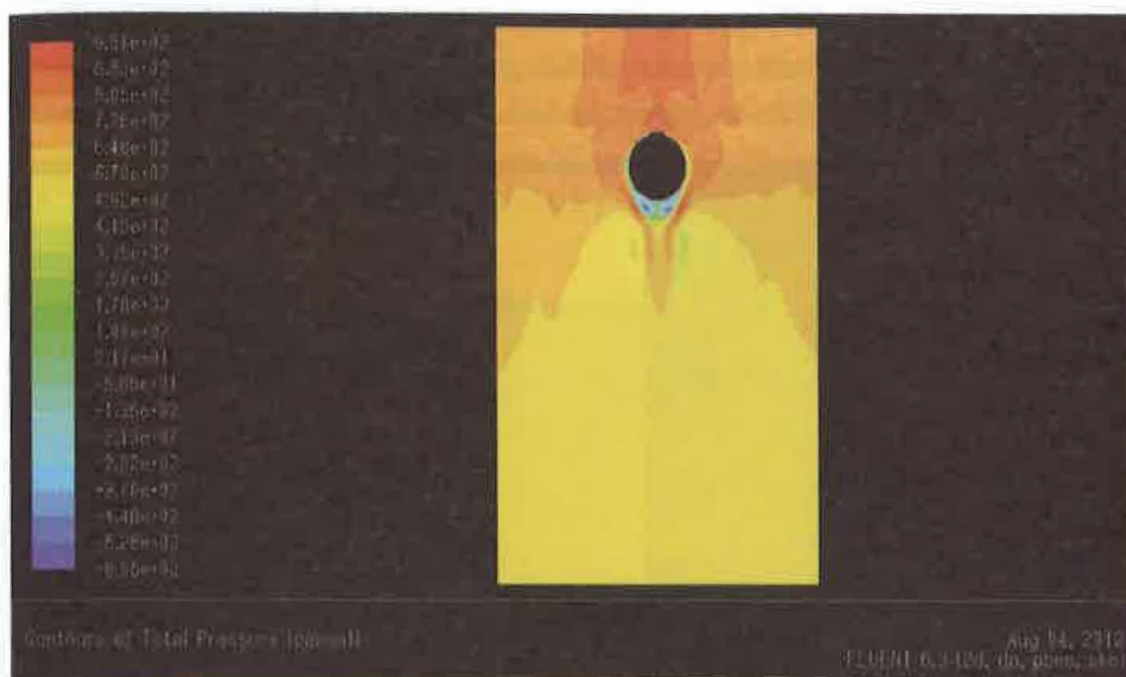
Figure 5: Total Predicted Pressure for seam angle 0^\circ
