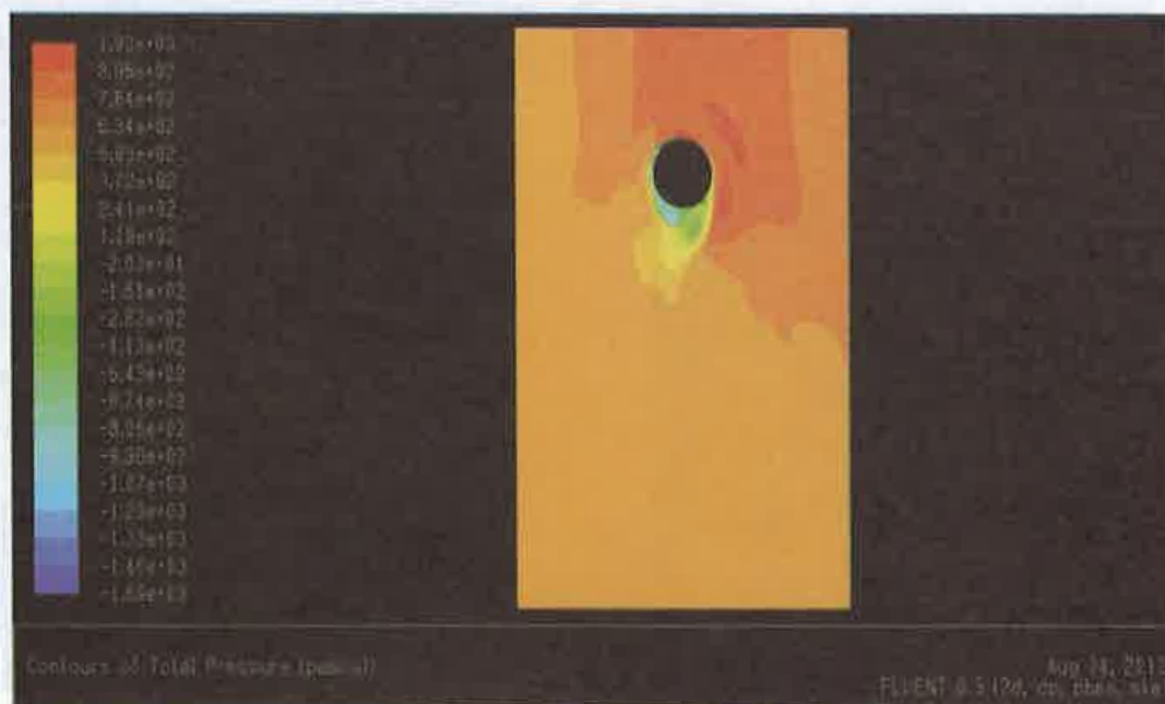
Figure 6: Total Predicted Pressure at seam angle 30^\circ for optimum conventional swing
