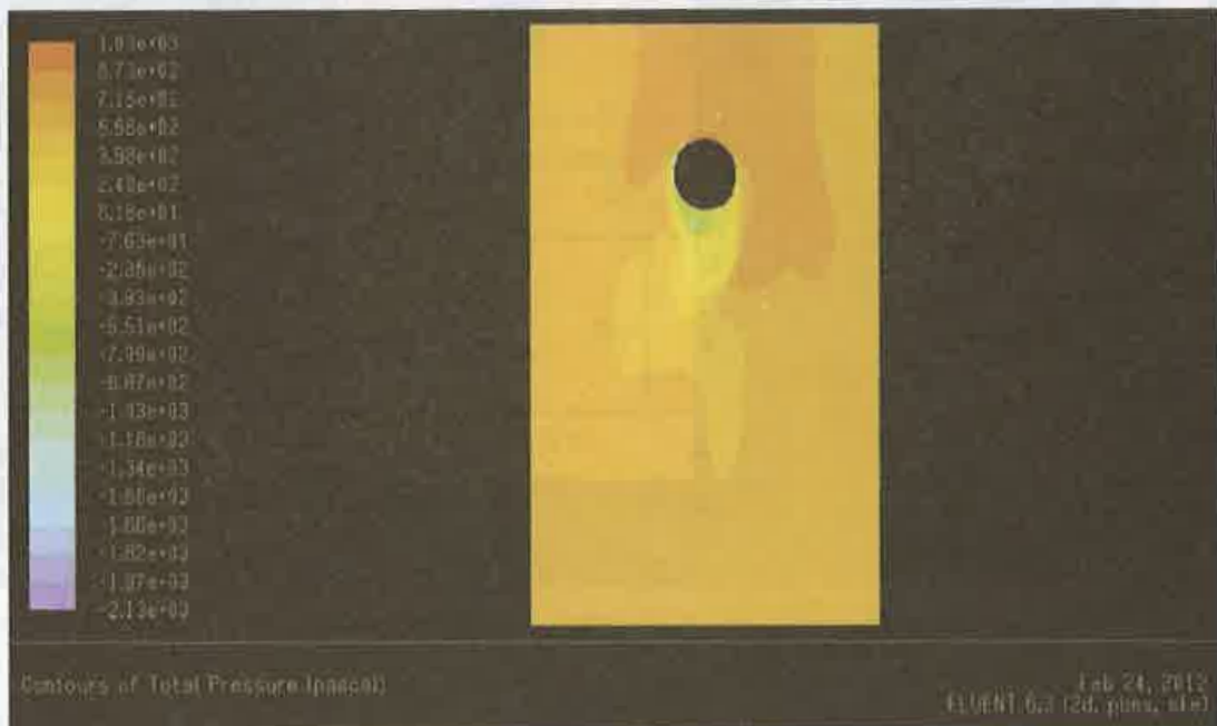
Figure 7: Total Predicted Pressure at seam angle 45^\circ for optimum conventional swing
