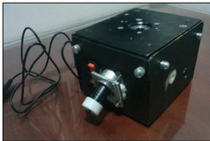
Figure 2. Box-shaped arrangement of the designed lubrication oil analyzer
