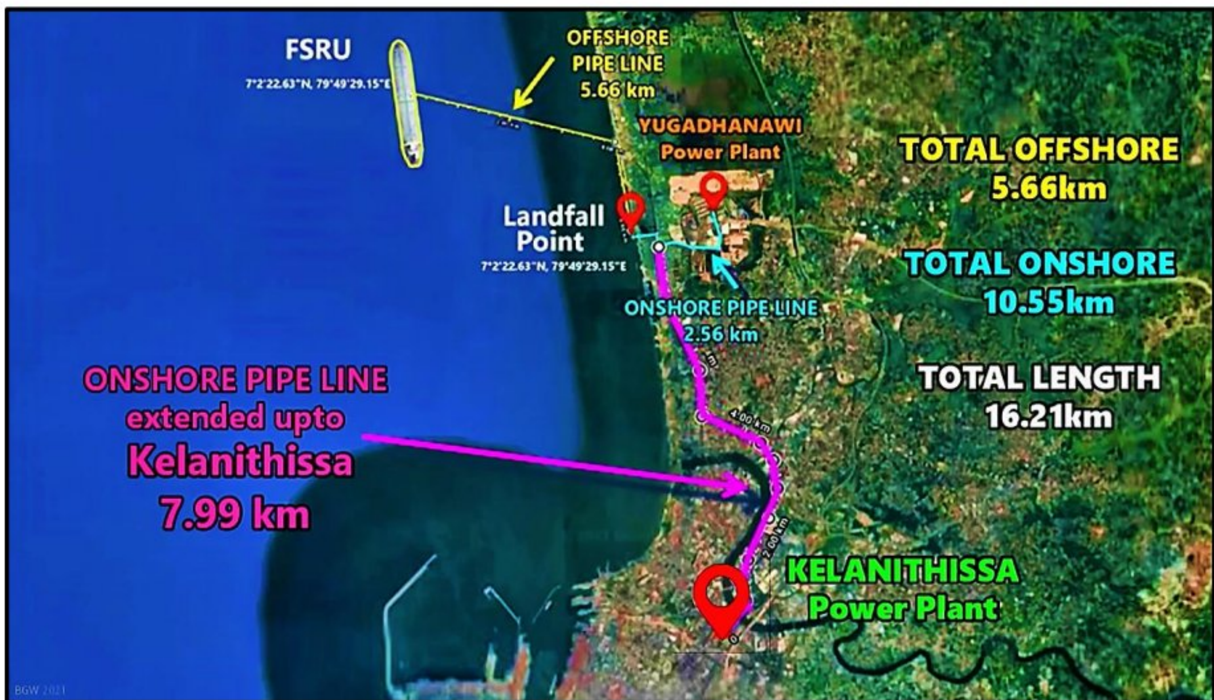
Figure 3.5 : Recommended Pipeline Route.
