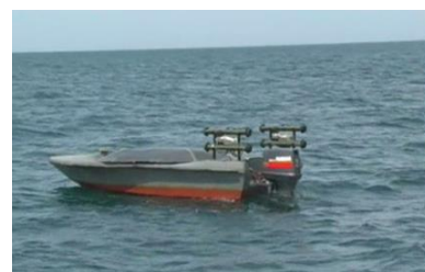
Figure 9. Prototype an explosive laden unmanned waterborne vehicle (initial testing)
