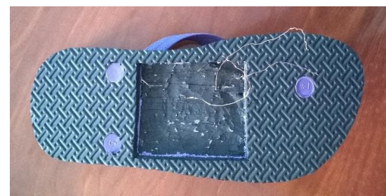
Figure 4: The cut on the underside of the slipper to made to accommodate the box and the wires drawn out from the sensors
