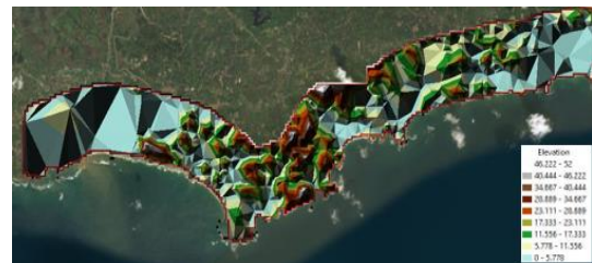
Figure 3. The Triangular Irregular Networks (TIN) model which developed for the Research area
