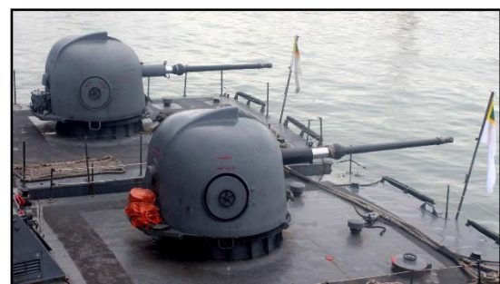
Figure 4: Oto Melara 76/62 mm Installed Onboard SLN FMVs
