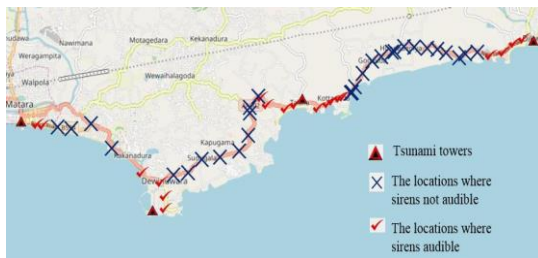
Figure 1. Locations of 4 Tsunami towers and locations of the interviewed points Source: Survey Department, Sri Lanka
