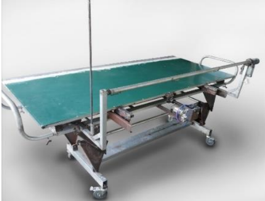
Figure 8. Lateral transferring unit with complete machine structure
