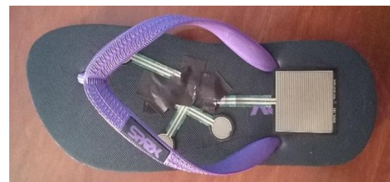
Figure 3: The placement of the sensors on the top surface of the slipper
