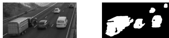
Figure 1: A grey-scale frame from a video sequence (left) together with the detected moving objects pixels image (right)
