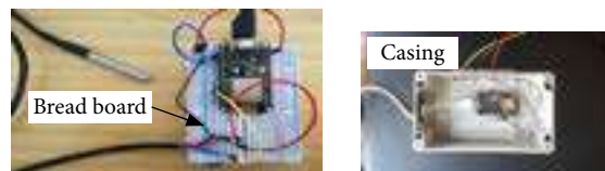
Figure 4. NodeMcu connected with temperature sensor and full setup with casing.
