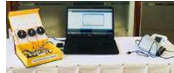
Figure 3. Initial Testing Prototype Model of the Braille Blood Pressure Reader developed on a breadboard using three Servomotors
