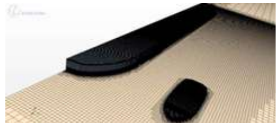
Figure 4: The final full scale 13.2 million CFD mesh model of the tug and ship.
