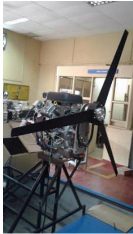
Figure 3: Engine mounted to the airboat
