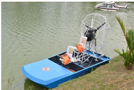
Figure 4: Seating arrangement of airboat
