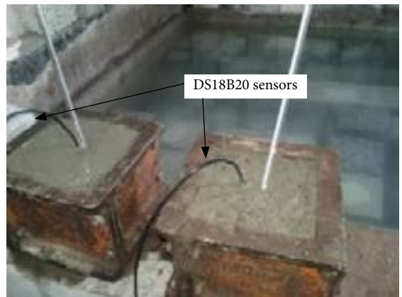
Figure 6. Laboratory test set up of monitoring temperature of samples using wireless system.
