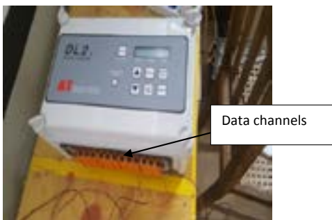
Figure 2: Typical data logging systems used in temperature monitoring.
