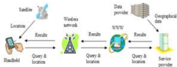
Fig 2 – How GPS location service works
