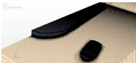
Figure 4: The final full scale 13.2 million CFD mesh model of the tug and ship.
