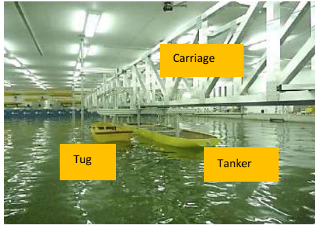
Figure 3: Experimental setup to measure the interaction effects between vessels in AMC's Model Test Basin
