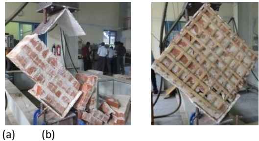
Figure 6: Wall panels at the end of the test; (a) Control wall panel (b) retrofitted wall panel
