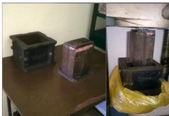
Figure 1: Tensile testing machine, concrete mould and mechanical attachment
