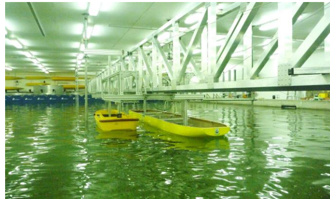
Figure 3. Experimental setup for interaction between vessels in AMC's Model Test Basin.
