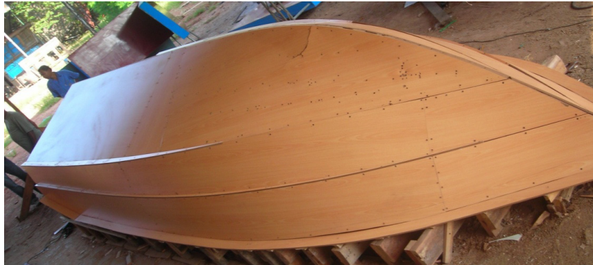
Fig C. Plug of the Boat Hull
