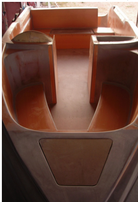
Fig D. Plug of the Deck
