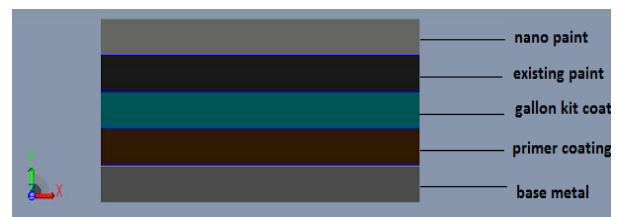
Figure 02: Solid works diagram for cross section of all coatings
