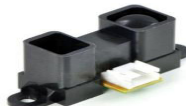
Fig 3. Sharp GP2Y0A02 sensor
